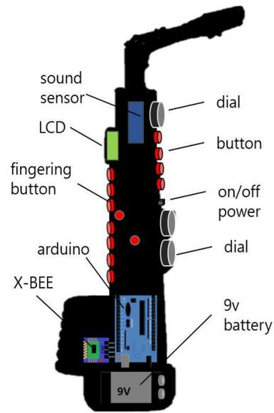
Figure 1. Structure and part of interface.
