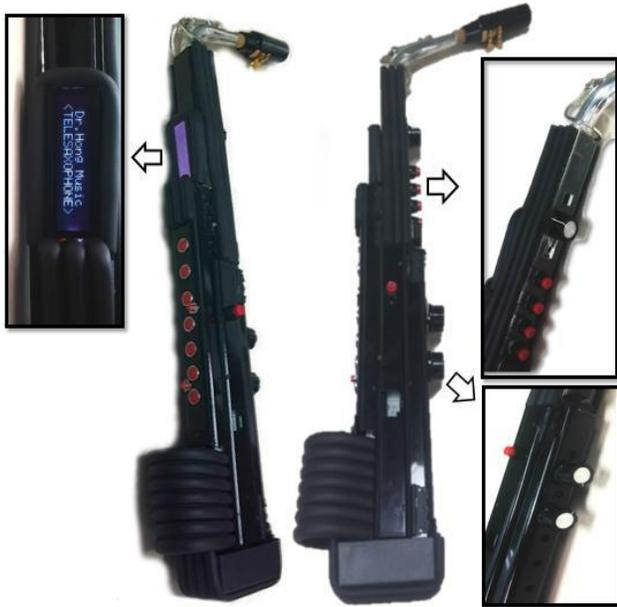
Figure 3. Display and sensors in Telesaxophone.
