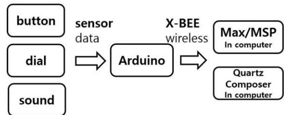
Figure 2. Data flow of the interface signals.
